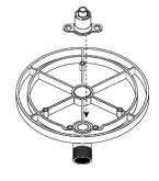
13) Fit drive gear, turn clockwise to secure.
